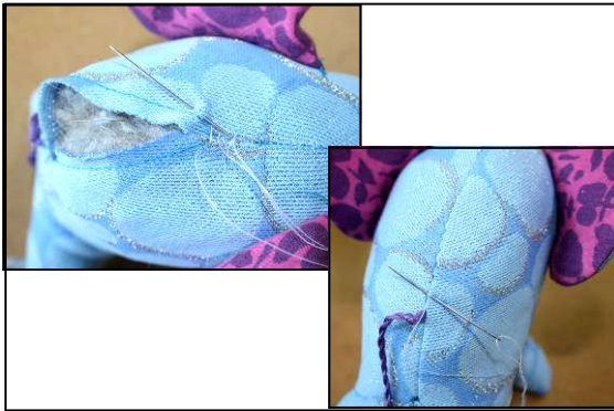
28. Hand stitch the opening closed with ladder stitch, using the stay-stitching as a guide.
