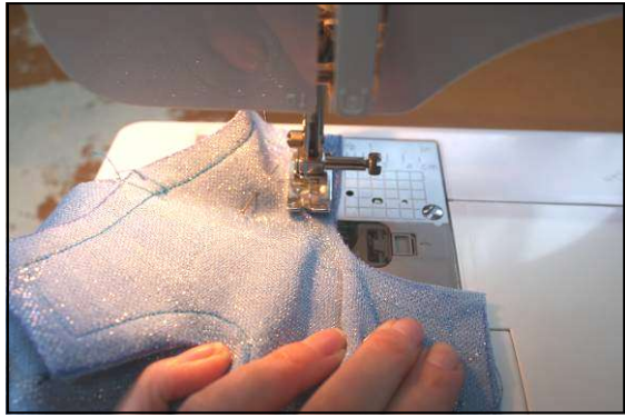
* To stitch around tight curves, stretch the fabric to open the curve out (and no speeding).
